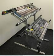
A standard unit is 1.5m in length and can be easily and securely be joined to form any length logging table.
